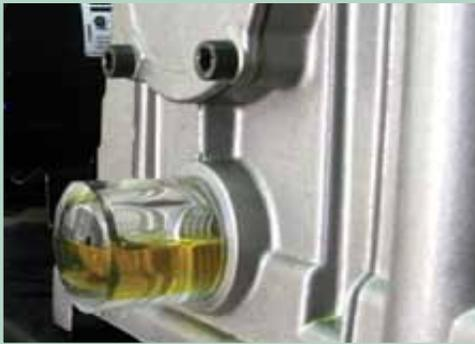
With Esco's 3-D BullsEye™, the reservoir oil can be inspected easily and accurately.
