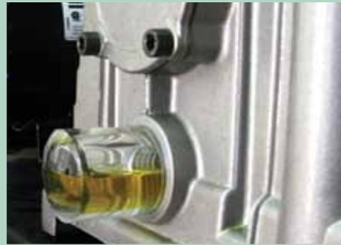
With Esco's 3-D BullsEye™, the reservoir oil can be inspected easily and accurately.
